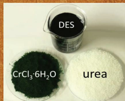
Figure 3: Solid tanning salt + solid urea makes a DES, a deep eutectic solvent.
